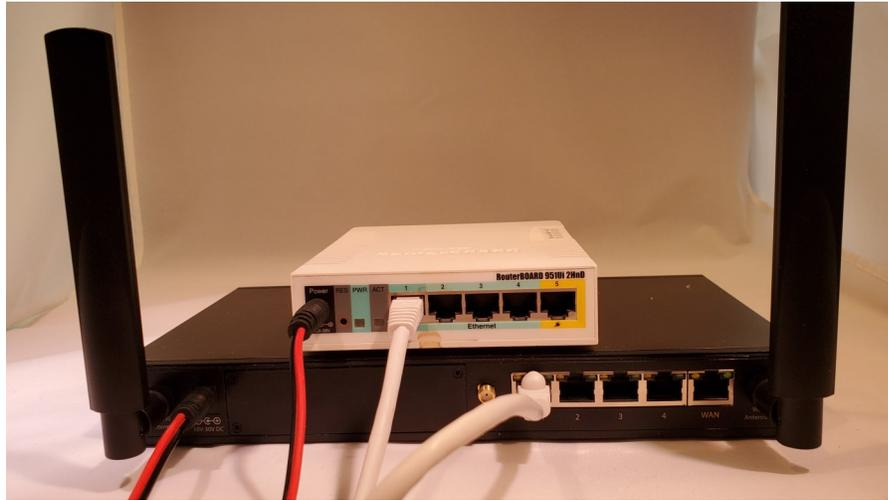
Cable connection between the IIM cell router and the IIMRB951: The orange or yellow ethernet cable connects to Port 1 on the IIMRB951 the other end of the orange or yellow cable connects to Ethernet port on IIM 2550-VAST. **Do not connect ethernet cable to port 5.**
